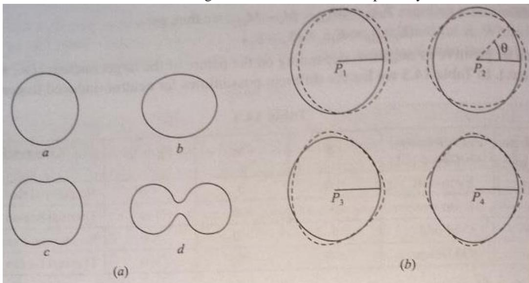
Fig. 3.1 (a) Various stages of deformation leading to the final splitting of a liquid drop. (b) Different modes of axially symmetric deformation of a liquid drop.
