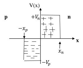
Due to diffusion of electrons from n-side to p- side and that of holes from p-side to n- side space charge is produced near the junction. Because of space charge variation near the junction an intrinsic potential barrier develops across the junction.
