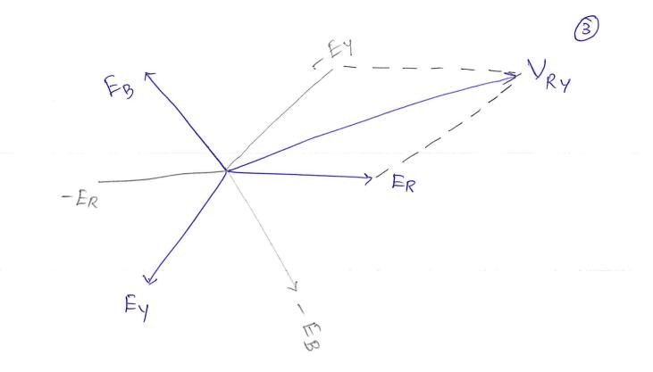
Apply KVL  $E_R - E_Y = V_{RV}$  $V_{RY} = \left( E_R^2 + E_Y^2 + 2 E_R E_Y \cos 60^{\circ} \right)$  $= \sqrt{E_p^2 + E_p^2} + 2 E_p E_p \cos 60'$ =  $\sqrt{3 E_p^2}$  $V_{Ry} = \sqrt{3} E_{P}$ Similarly  $E_Y - E_B = V_{YB} \implies V_{YB} = \sqrt{3} E_p$  $E_{B} - E_{R} = V_{BR}$  $\Rightarrow$   $V_{BR} = \sqrt{3} E_p$
