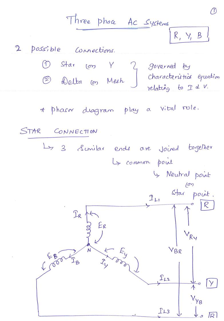
$$T_{R}, T_{V}, T_{B} \rightarrow Phase Currents.$$
