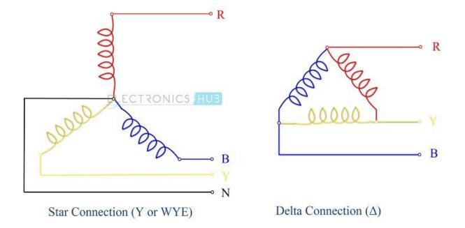
Let us understand more about these connections by using the following Comparison between Star and Delta Connections.
