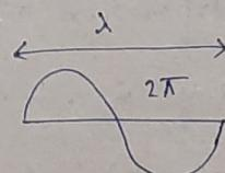
$$\begin{aligned}\delta_2 &= \frac{2\pi}{\lambda} \times \text{path difference} \\ &\quad \text{between two waves} \\ &= \frac{2\pi}{\lambda} n\end{aligned}$$
