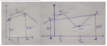
The Lagrange's M.V.T states that between two points A and B of the graph of the function f there exists at least one point where the tangent is parallel to the chord  $\overline{AB}$ .
