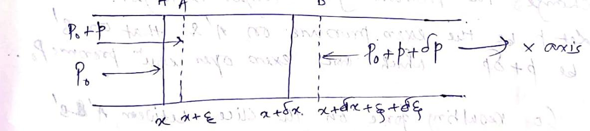
Let us consider a tube of fluid of unit cross-section with its axis in the direction of propagation of the wave. Two planes A & B are at  $x$  &  $x + \delta x$  initially. Such that  $\delta x \ll \lambda$  and  $\delta x \gg$  mean molecular separation.
